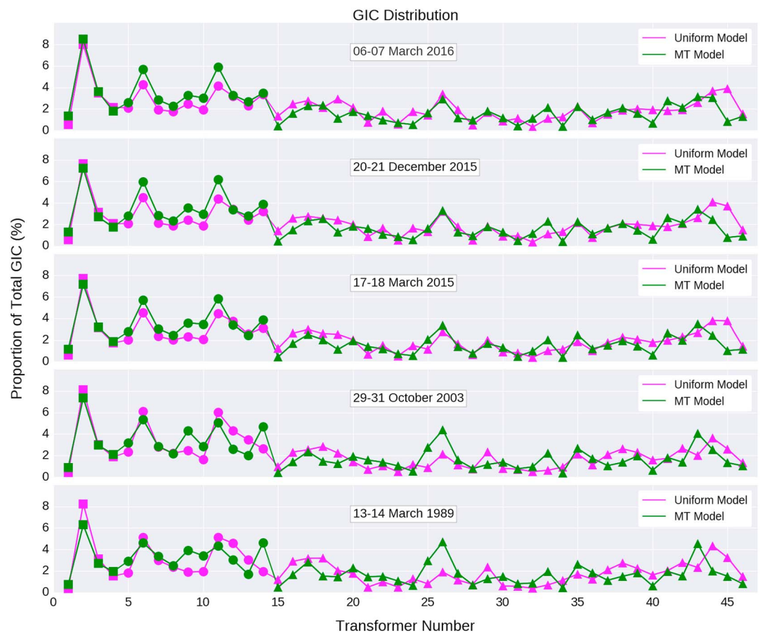
Figure 7. Distribution of total GIC in the Irish power network for each of the events in this paper as calculated using the homogenous and MT resistivity models. (first to fifth panels) Events are listed in reverse chronological order. Squares, circles, and triangles represent 400 kV, 275 kV, and 220 kV transformers, respectively. Transformer number indicates the transformer seen in Figure 3.
